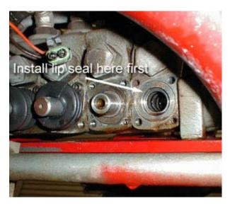
With the whole valve shaft out, it's real simple to change the retaining washer and backup seal, without even touching the springs. With it out, it's a great time to insert the lip seal in the valve bank, then push the valve shaft back up in place. The shaft does have a top and bottom, be careful.
