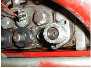
This is with the cover removed. First time I had to change one of these I then unscrewed the end of the valve shaft with the spring retainers. Which basically opened a 3/8 hole to the hydraulic tank. At least that's what it felt like when the spring took off with the end piece and I'm laying under it with my thumb plugging the hole wondering what I'd gotten myself into. The next time I did this I drained the tank first, but it was still a chore to do.
